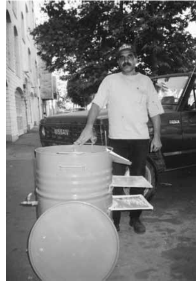
Slightly modified version of "Ankara Flotation" device and its builder Mr. Jafar Sfidari. Device will be used to retrieve carbonized seeds and other plant remains
